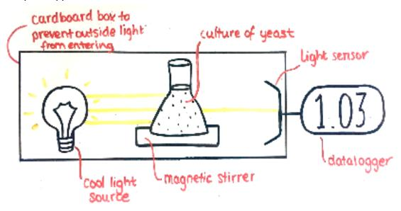
2. Leave the datalogger to continuously record absorbance readings for 12 hours.
